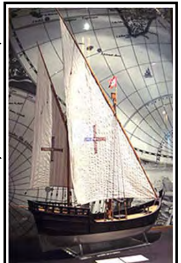
Portuguese caravel. The caravel was developed by the Portuguese for use in the 15 th Centruy. This was the standard model used by the Portuguese in their voyages of exploration. It was able to sail into the wind, unlike every other ship.
